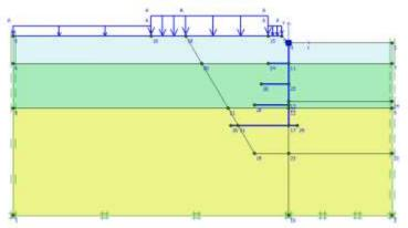
Figure 4 - Modeling retaining wall with heel in PLAXIS software
