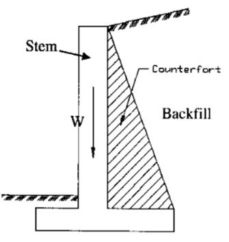
figure1-Diagram of a counterfort wall
