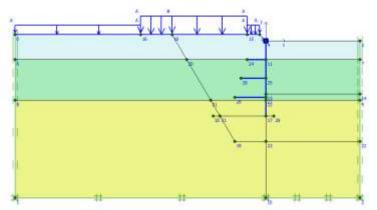
Figure 5 - Modeling retaining wall without heel in PLAXIS software
